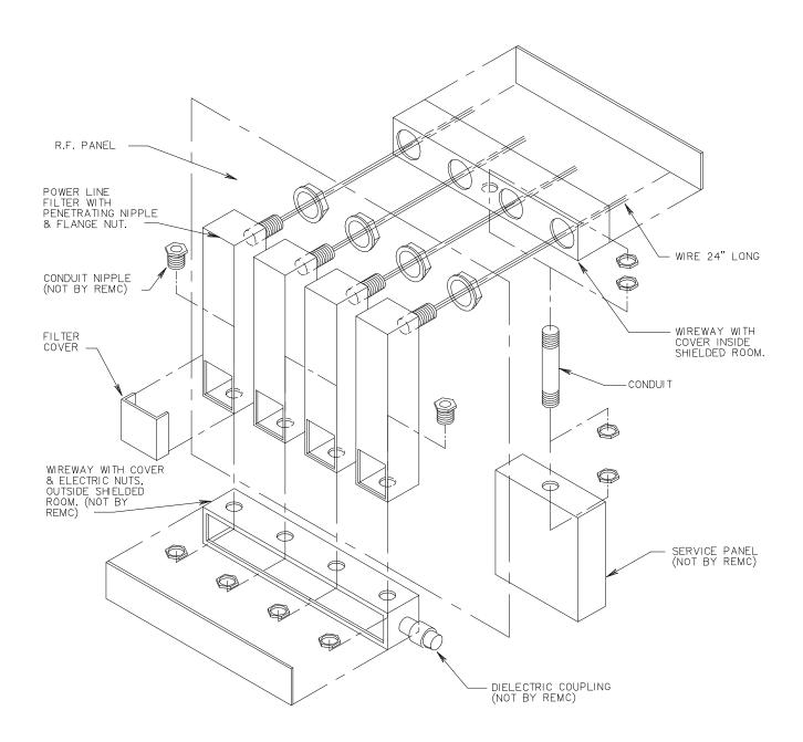
NOTE: RAYMOND EMC PROVIDES FILTER UNITS WITH FLANGE NUTS.
